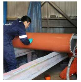
Thermal insulation barrier providing corrosion protection with "cool-to-touch" properties
